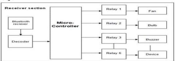
Fig 1.1 block diagram of home automation system
